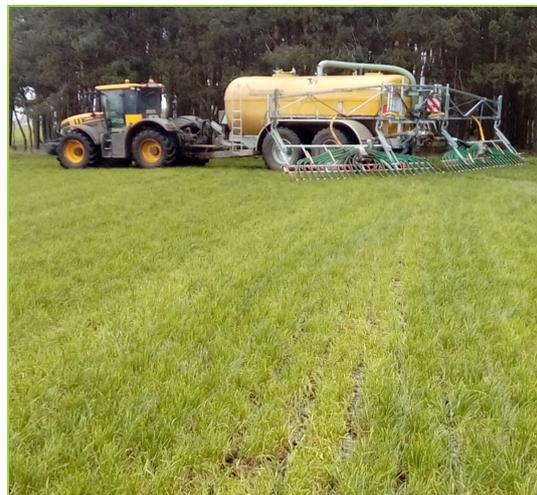
The main reason that induced farmers to choose this kind of equipment was that manure is not spread over the grass but goes directly into ground. In this solution slurry is pumped from a tank and is injected via drag hose directly on the soil surface. Innovative electronic solutions allows for all data to be recorded and saved. During application it can be distributed fully automatically and exactly according to the desired N
